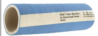
TR2 is a rubber covered, smooth bore FEP hose, available up to 3" diameters. It handles a very broad range of chemicals and has an abrasion, weather, and ozone resistant blue EPDM cover. Other colors available.
